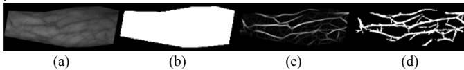
Fig. 13 Illustration of the ROI and the vein area size. (a) a segmented NIR image, (b) its ROI, (c) the enhanced vein pattern from (a), and (d) the binarized vein pattern from (c). The number of white pixels in (b) represents the size of ROI and the number of white pixels in (d) represents the size of the vein pattern.
