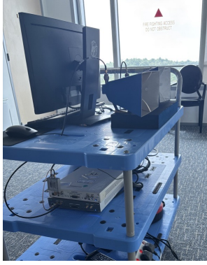
Fig. 3. Photo of our SDR-based CW radar station #2
