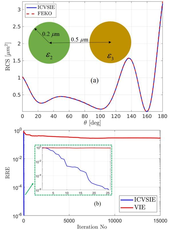
Fig. 2. (a) The RCS computed using the proposed ICVSIE method and the FEKO. (b) The number of iterations versus RREs obtained during the iterative solutions of ICVSIE and VIE systems.
