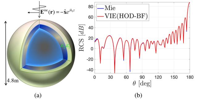
Fig. 1. (a) Two-layered shell with  $\epsilon_1 = 2\epsilon_0$ , and  $\epsilon_2 = 4\epsilon_0$ . (b) The RCSs computed with the proposed solver and Mie series solution at  $f = 600$  MHz.
