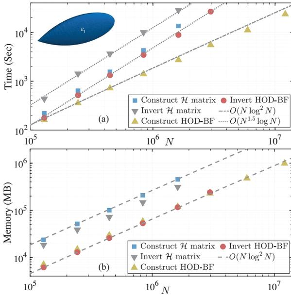
Fig. 2. (a) CPU and (b) memory scaling of the HOD-BF-accelerated solver and  $\mathcal{H}$  matrix-accelerated solver when applied to the EM analysis of a NASA almond with permittivity  $\epsilon(\mathbf{r}) = (4 - 0.0001j) \epsilon_0$
