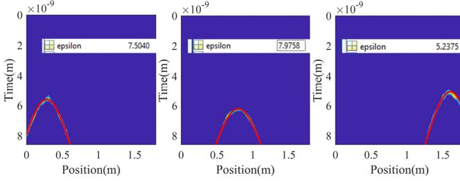
Fig. 3. The extracted hyperbolae corresponding to three roots and the estimated relative permittivity of the surrounding soil of each root.
