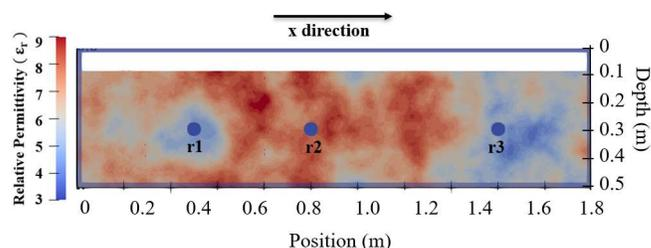
Fig. 1. Side view of the simulation scenario, where r1 to r3 are cylinders representing three roots. The soil’s relative permittivity values around r1, r2, r3 are significantly different from each other.
