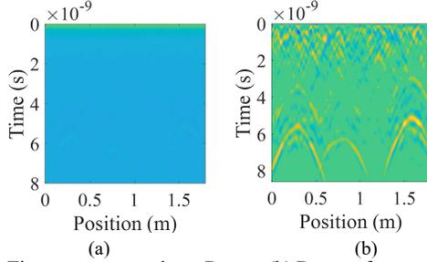
Fig. 2. (a) Time-zero corrected raw B-scan. (b) B-scan after pre-processing techniques.
