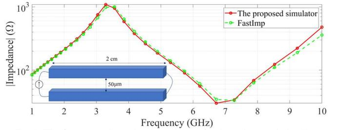
Fig. 1. The frequency-dependent impedance of a shorted transmission line
