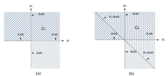
Fig. 3 Illustration of a non-unique representation of a convex polyhedral cone and a redundant constraint. (a) the convex polyhedral cone  $C_1$  defined by Eq. 5 and (b) the convex polyhedral cone  $C_2$  defined by Eq. 6.
