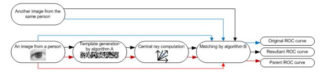
Fig. 10 Illustration of three different matching processes. The blue, black and red arrows indicate respectively the processes of computing genuine matching scores for original, resultant and parent ROC curves.
