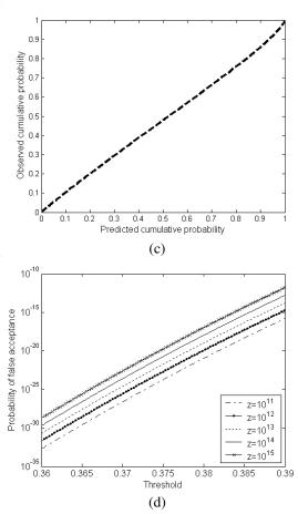
Fig. 4 Model validation and predications (a) empirical and theoretical distributions from non-translated matchings, (b) a plot of predicted cumulative probability against observed cumulative probability for non-translated matchings, (c) a plot of predicted cumulative probability against observed cumulative probability for translated matching and (d) the probability of false acceptances against different thresholds.
