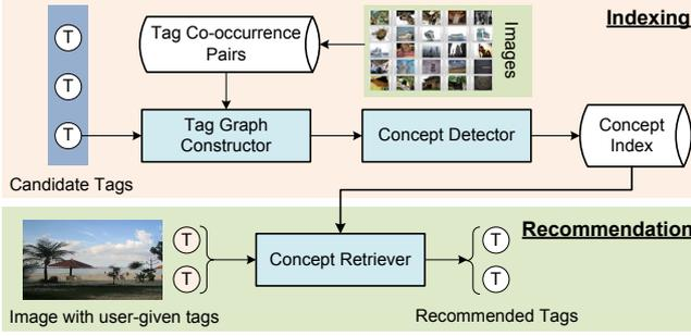
Figure 2: Architecture of the tag recommendation system.
