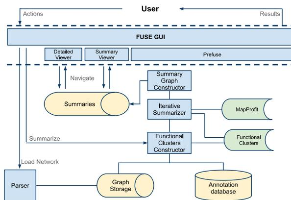
Figure 2: Architecture of FUSE.
