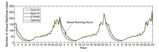
Fig. 4. Performance of different dispatching algorithms for a sample period of 3 days
