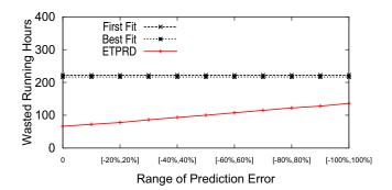
Fig. 7. Performance for different prediction errors
