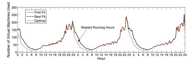
Fig. 3. Performance of First Fit and Best Fit dispatching for a sample period of 3 days
