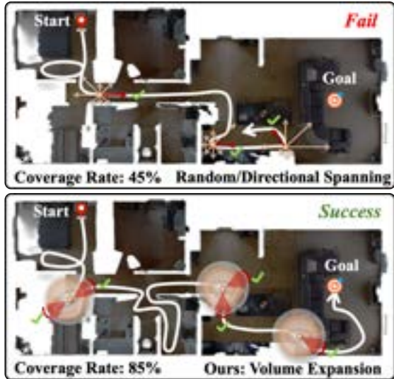
Figure 1. Embodied navigation task: Top: Random/directional spanning repeatedly probes directions that are infeasible under environment and dynamics constraints, causing local cycling and getting stuck, which limits exploration ( 45% coverage ) and fails to reach the goal. Bottom: Our volume expansion objective prioritizes low-covered reachable directions, yielding broader exploration ( 85% coverage ) and successfully reaching the goal.
