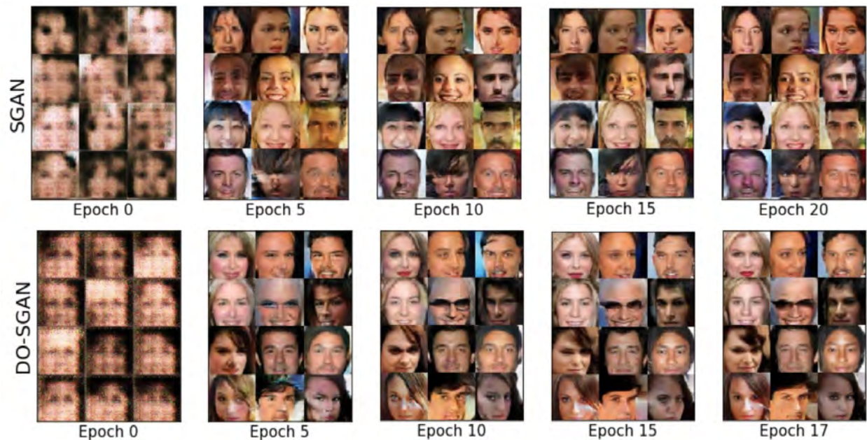
Figure 5.1: Training images with fixed noise for SGAN and DO-SGAN/P (pruning) until termination. Both during training and after convergence, DO-SGAN/P can generate better quality images with FID score of 6.32 against SGAN’s FID score of 6.98.
