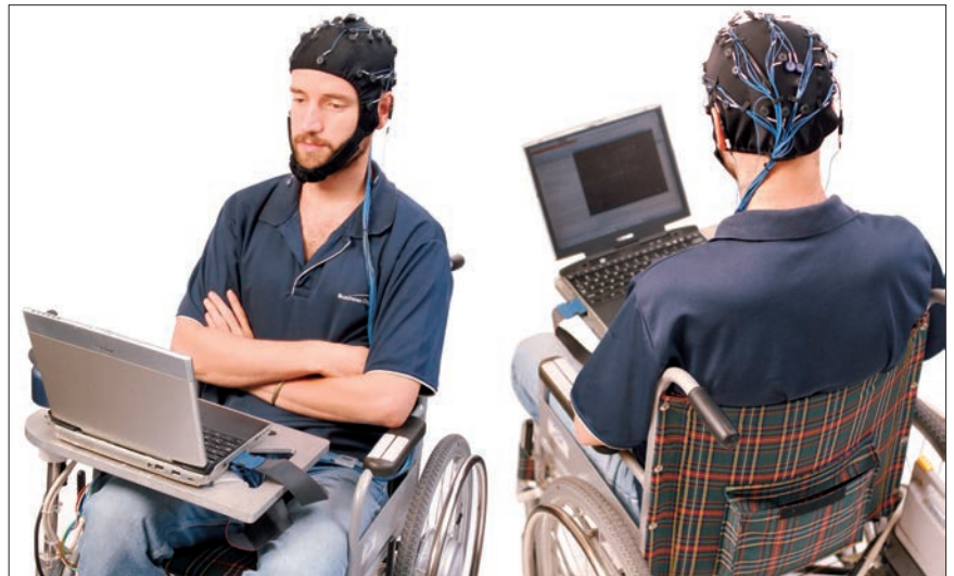
Figure 1. The brain-controlled wheelchair uses a compact acquisition device and an embedded computer.
