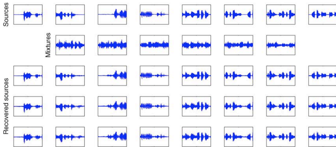
Fig. 3. Separation results in Example 3. The first row: eight speech sources; the second row: six mixtures; the third row: eight recovered sources based on a seven-level WPT; the fourth row: eight recovered sources based on a one-level WPT; the fifth row: eight recovered sources based on sparse representation in the time domain (without WPT).
