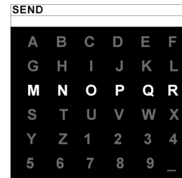
Fig. 1. Interface of a P300-based word speller: Six rows and six columns shown above flash alternatively in a random order during each flashing round. A P300 event-related potential (ERP) will be elicited when the row or the column specifying the focused cell flashes. The row and the column specifying the focused cell can be determined through the identification of P300 ERP within the EEG recorded during the flashing process.
