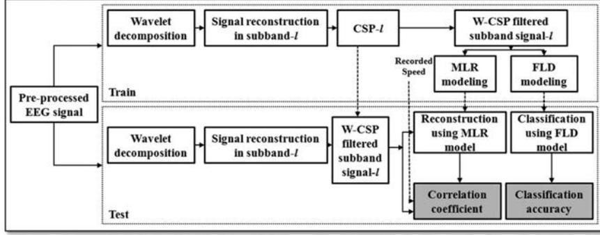
Fig. 3. Proposed wavelet-CSP algorithm.
