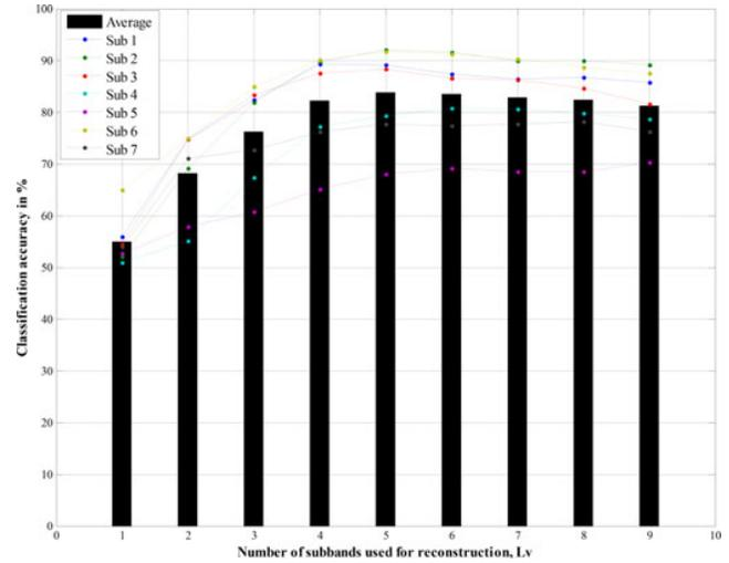
Fig. 5. Effect of using different number of subbands for classification. The results are for speed classification (fast versus slow movement).
