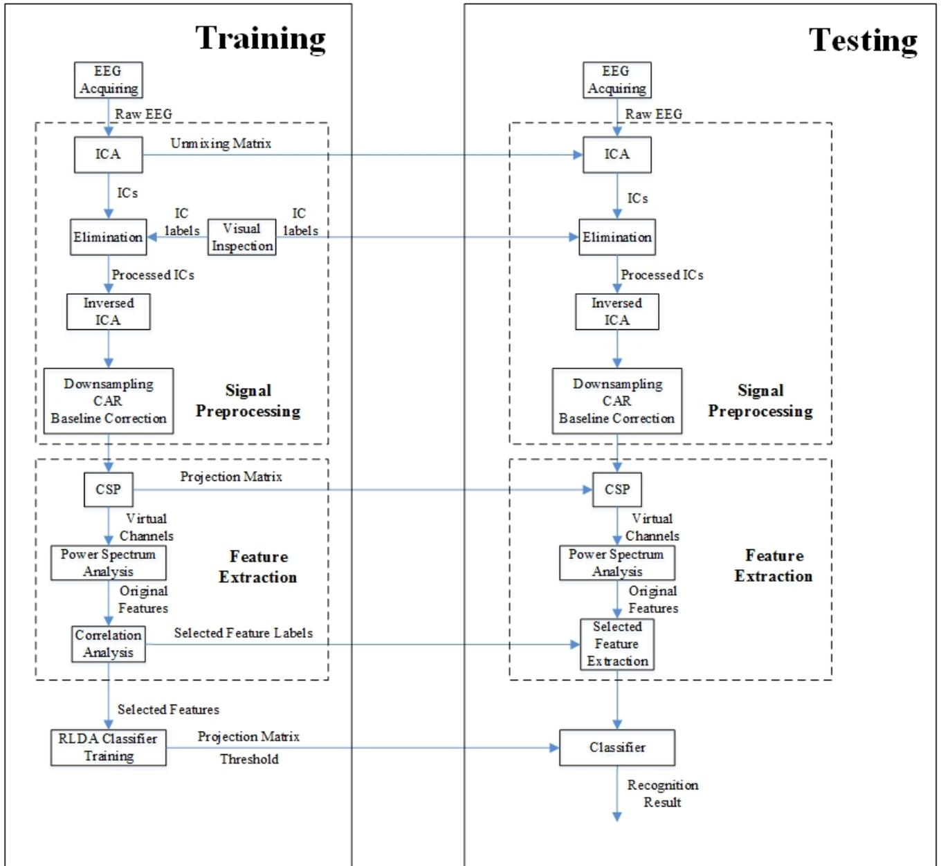
Fig. 3. Flowchart of Intention Decoding Algorithm (IDA)
