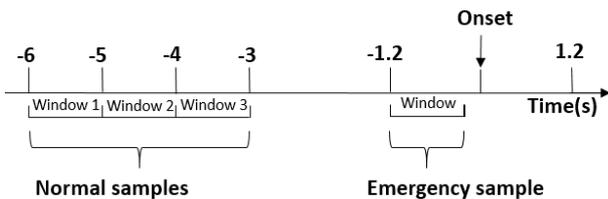
Fig. 4. Extraction of normal samples and emergency samples for training
