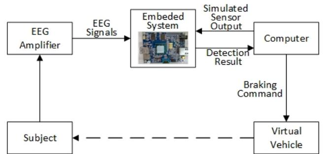
Fig. 8. Structure of real-time detection system
