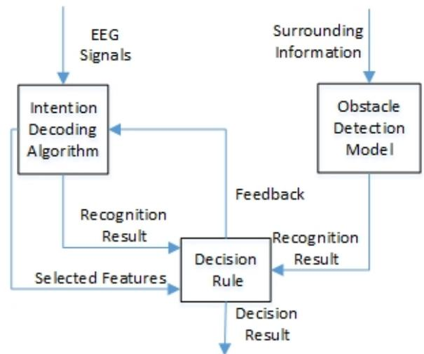
Fig. 2. Architecture of the whole emergency situation detection system
