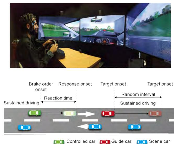
Fig. 1. The experimental setup and protocol.
