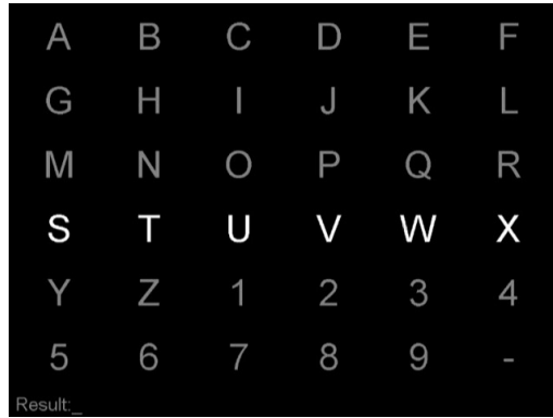
Figure 1. P300 Speller Display. Rows and columns are highlighted randomly and are repeated several rounds. The picture shows the 4 th row is intensified.
