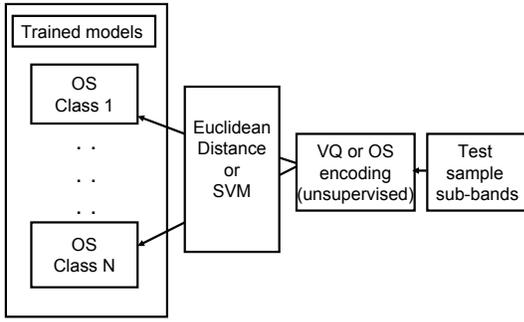
Fig. 2. Proposed non-parametric statistical encoding and testing.
