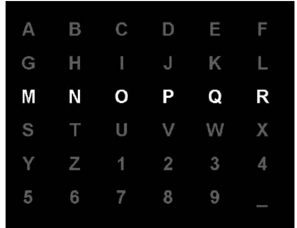
Fig.1 The stimulus matrix shown to the user. One of the rows or one of the columns of the matrix was intensified.
