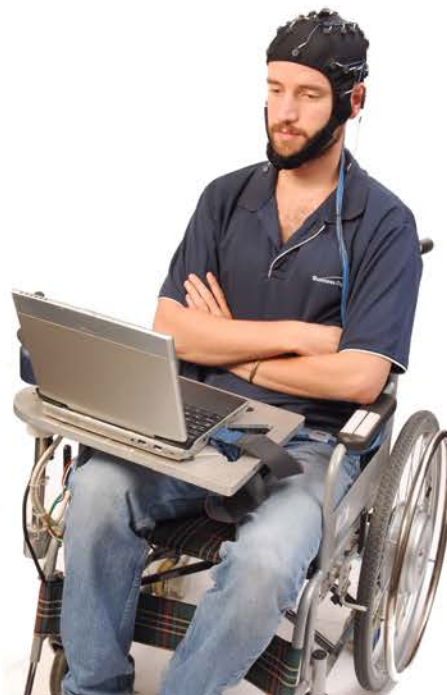
Fig. 1. Photograph of the prototype wheelchair controlled by thought, which can move in a building environment.
