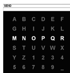
Figure 1. Interface of P300-based speller.
