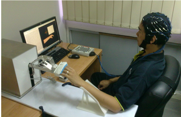
Fig. 1. Experimental setup to collect EEG data from passive movement of the left hand using the haptic knob robot [17] for calibrating EEG-based motor imagery BCI.
