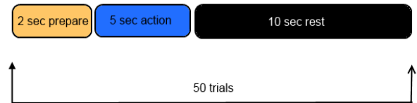
Figure 3. Experimental protocol design for multimodal NIRS and EEG-based motor imagery BCI. Action is motor imagery or idle in motor imagery run and passive movement or idle in passive movement run.
