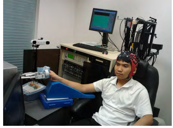
Figure 2. The multi-modal NIRS+EEG experiment setup for subject performing motor imagery and passive movement using the haptic knob.
