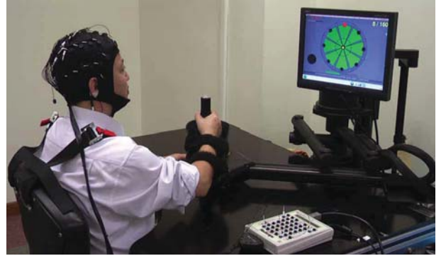
Fig. 4. Setup of EEG-based motor imagery BCI with robotic feedback rehabilitation for stroke.
