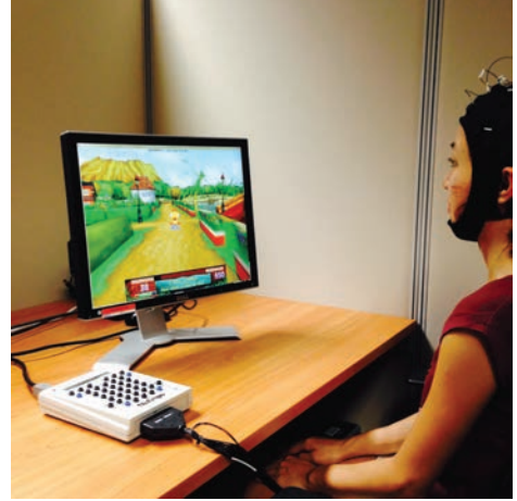
Fig. 2: Experimental setup to collect EEG data during NF training sessions. Subjects should modulate their brain signals to move the avatar on the screen.
