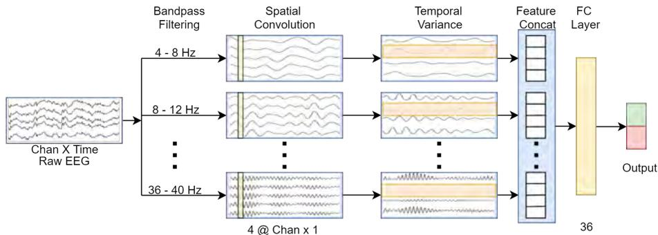
Fig. 1. Proposed network architecture: FBCNet.
