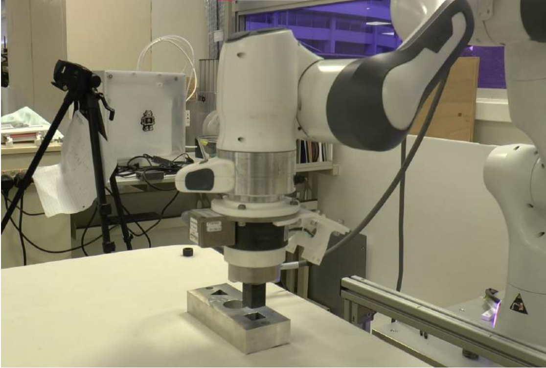
FIGURE 4.1: Robotic assembly setup. A square peg was used in this study.
