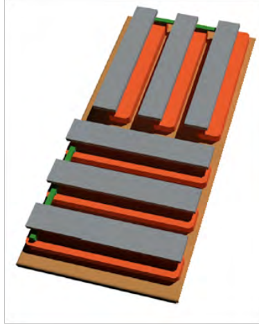
Figure 4.21: Physical structure of orthogonal multi-finger pixels.
