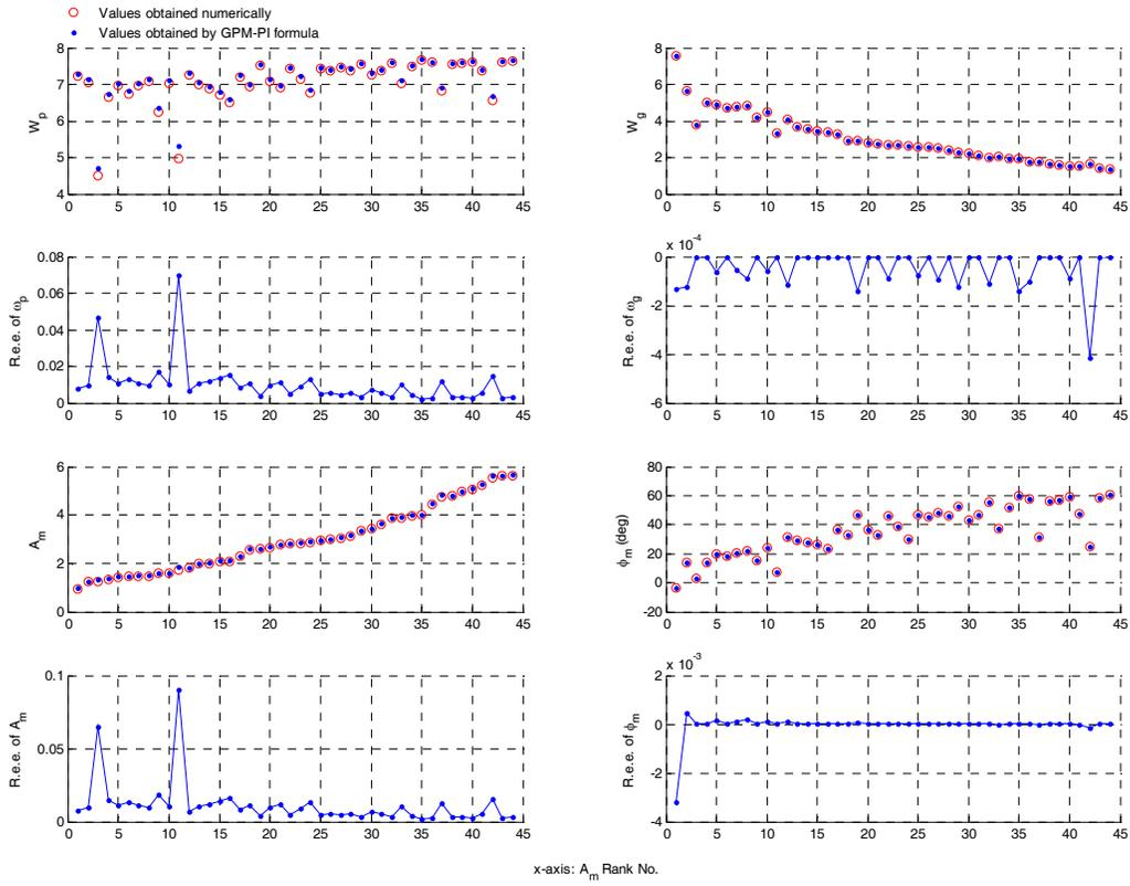
Fig. 2. The realized GPM of the PI tuning formulas in Table 1: comparisons between the GPM numerically obtained by MATLAB function “margin” (taken as the true GPM) and those estimated by the *GPM-PI formula* [2]. The relative estimation error (R.e.e.) is defined as  $R.e.e. := (the\ estimated\ value - the\ true\ value) / the\ true\ value$ .
