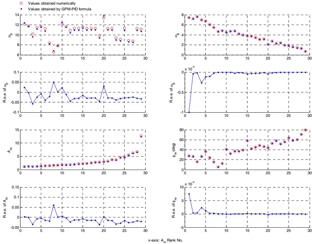
Fig. 4. The realized GPM of the PID tuning formulas in Table 3: comparisons between the GPM numerically obtained by MATLAB function “margin” (taken as the true GPM) and those estimated by the *GPM-PID formula* [2]. R.e.e. is defined the same as that in Fig. 2.
