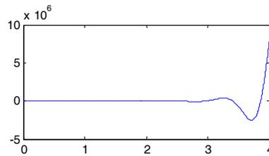
Fig. 6. Step response of an exemplary PI control system: the IPTD process is  $G_p(s) = 100e^{-0.2s}/s$  and the controller is tuned by the rule “Minimum ISE – Hazebroek and Van der Waerden (1950)” as presented in Table 1. The divergent response indicates the instability of the rule, justifying its realized gain margin of  $A_m < 1$ .
