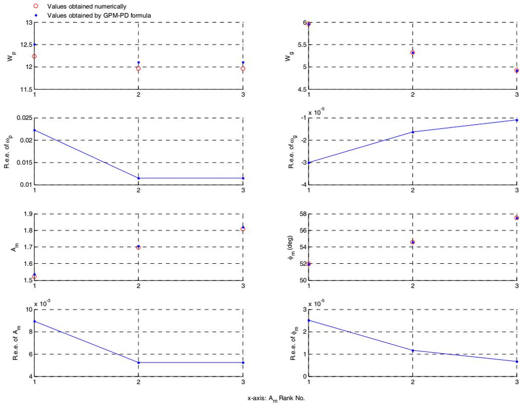
Fig. 3. The realized GPM of the PD tuning formulas in Table 2: comparisons between the GPM numerically obtained by MATLAB function “margin” (taken as the true GPM) and those estimated by the *GPM-PD formula* [2]. R.e.e. is defined the same as that in Fig. 2.
