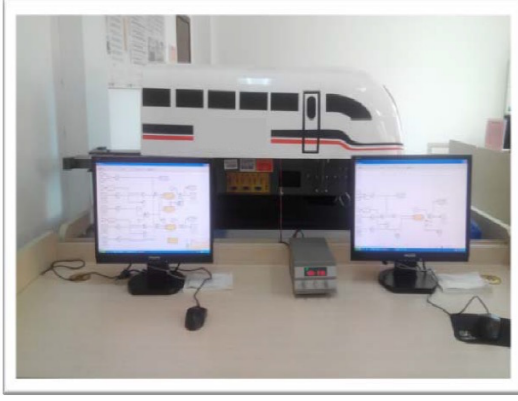
Fig. 5. Experimental platform of the maglev train.
