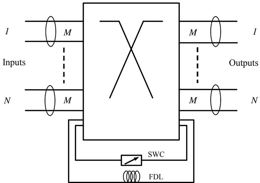
Fig. 3: Typical OPS configuration with SWCs and FDLs.
