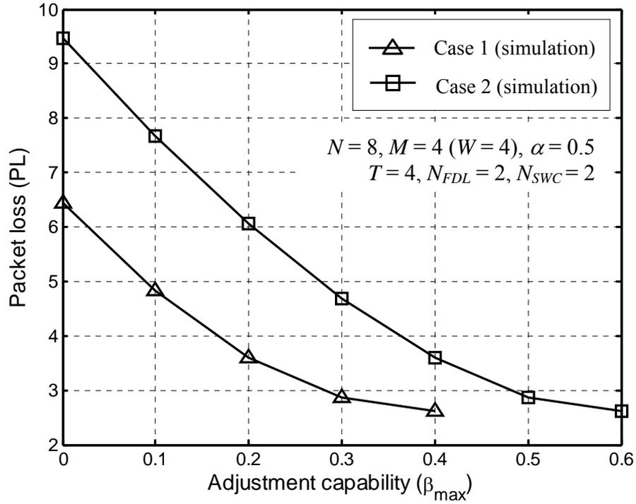
Fig. 10: Performance of the LB algorithm in OPS with both FDLs and SWCs ( $N_{FDL} = 2$ ,  $N_{SWC} = 2$ ). Traffic allocation adjustments are made in time dimension (uniform traffic pattern).
