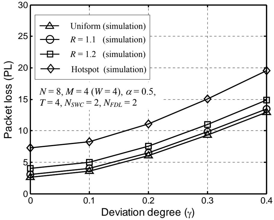
Fig. 6: Packet-loss performance in the OPS with both SWCs and FDLs.
