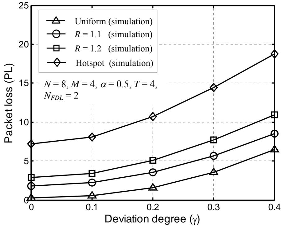
Fig. 4: Packet-loss performance in the OPS with FDLs but no SWC.
