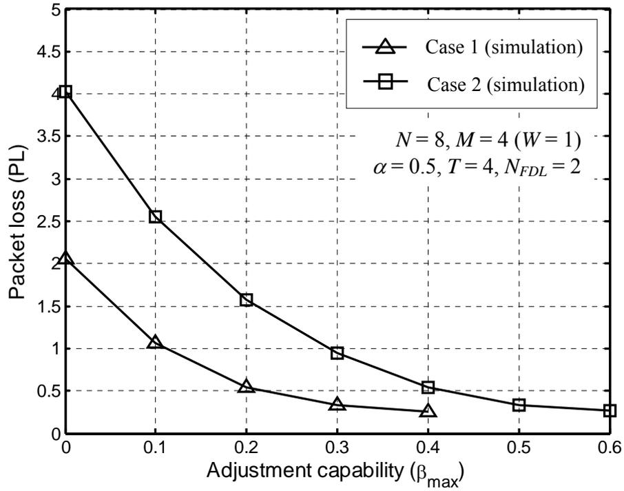
Fig. 8: Performance of the LB algorithm in OPS with only FDLs ( $N_{FDL} = 2$ ). Traffic allocation adjustments are made in time dimension (uniform traffic pattern).
