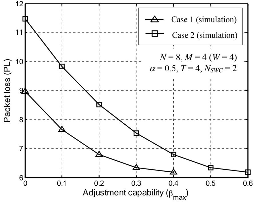
Fig. 9: Performance of the LB algorithm in OPS with only SWCs. ( $N_{SWC} = 2$ ). Traffic allocation adjustments are made in time dimension (uniform traffic pattern).
