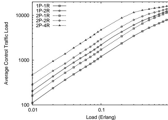
Fig. 13. The average number of control messages processed every second in PacNet under traffic with an average duration of connection of 100 ms.
