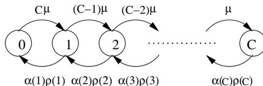
Fig. 2. The birth-death process of different link states in wavelength-routed networks with distributed parallel reservations.
