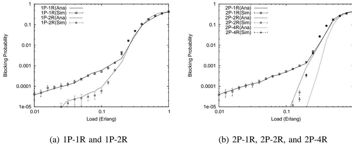
Fig. 12. Accuracy of the analytical models in 12-node ring under short-duration traffic with an average duration of connection of 100 ms. There are 16 wavelengths in each fiber.
