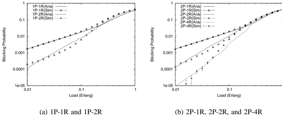
Fig. 10. Accuracy of the analytical models in PacNet under extra short-duration traffic with an average duration of connection of 10 ms.
