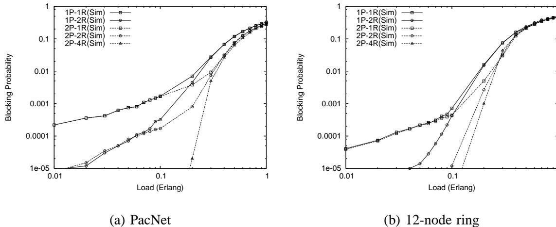
Fig. 4. Blocking performance of the different parallel reservations schemes under traffic with an average duration of connection of 100 ms.
