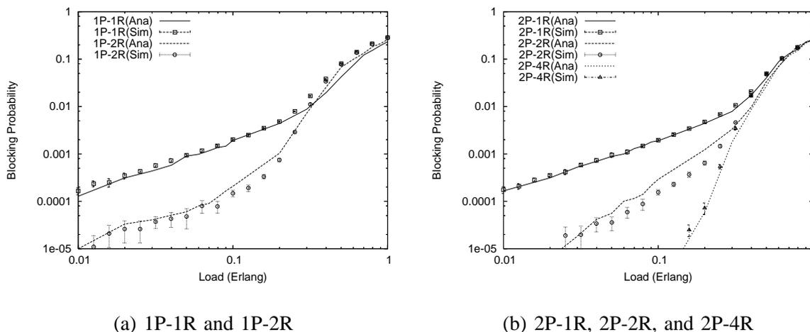
Fig. 11. Accuracy of the analytical models in PacNet under short-duration traffic with an average duration of connection of 100 ms. There are 16 wavelengths in each fiber.
