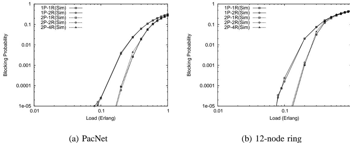
Fig. 5. Blocking performance of different parallel reservations schemes under traffic loads with an average duration of each connection of 1000 s.
