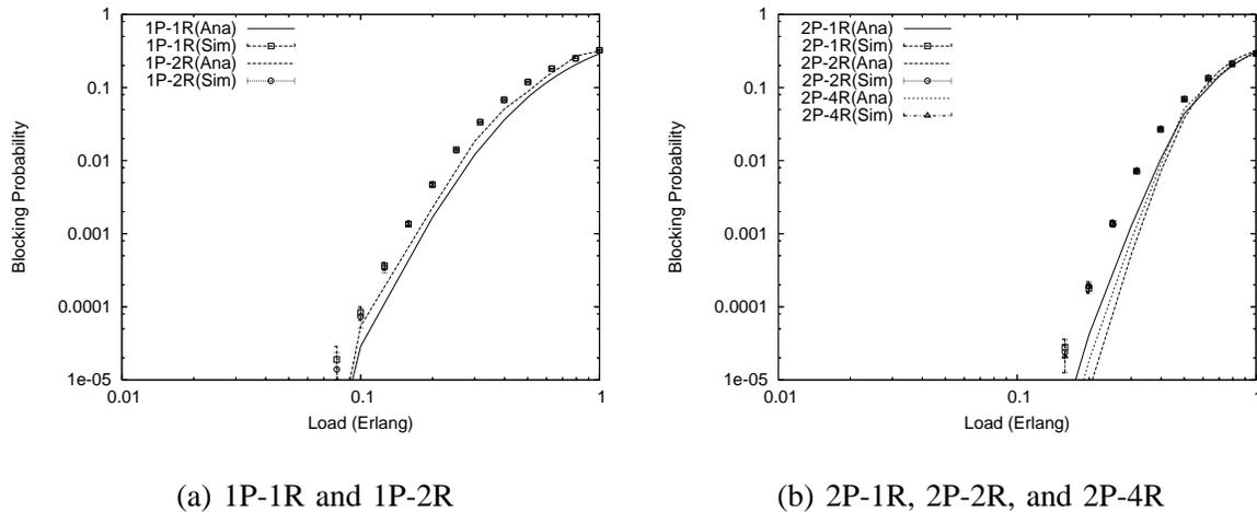
Fig. 8. Accuracy of the analytical models in PacNet under long-duration traffic with an average duration of connection of 1000 s.
