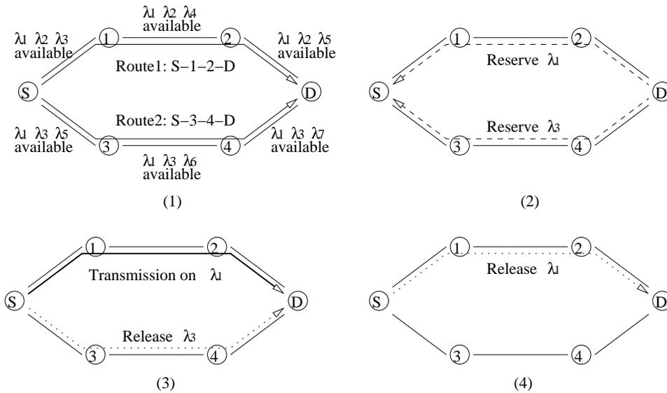
Fig. 1. An example of the MPPR scheme where we have two candidate routes and one reservation on each route (i.e., the 2P-2R scheme).
