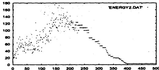
Fig. 1 Time evolution of the discrete energy function for 10 city TSP with Chen and Aihara's Method.
