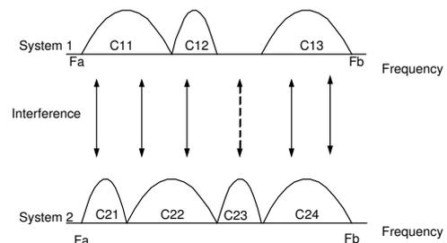
Fig. 1. Cochannel interference model for two adjacent satellite communications systems.
