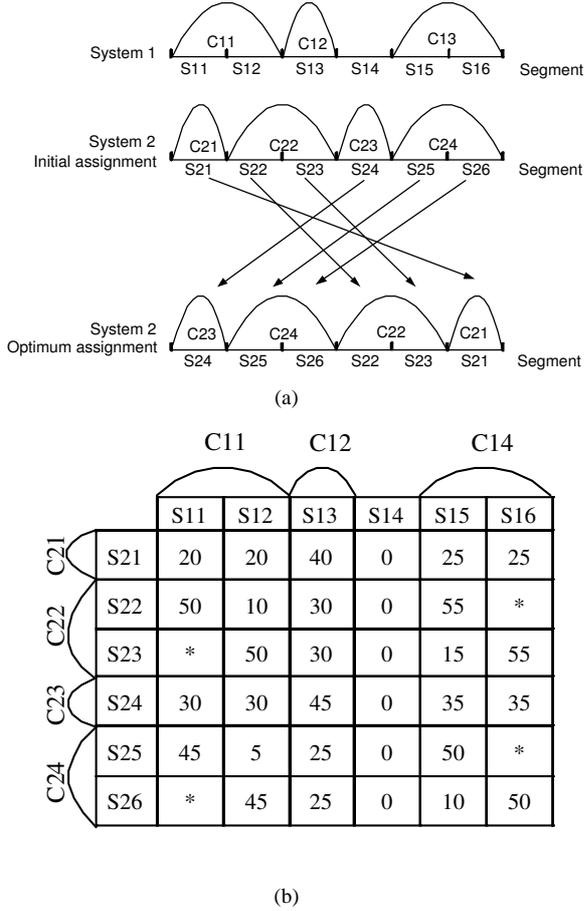
Fig. 2. Segmentation and interference matrix for the system in Fig. 1. (a) Segmentation of the two systems. (b) the interference matrix for the  $M$ -segment system.
