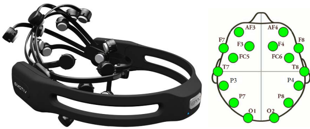
Fig. 3. The Emotiv EEG Device used in this study and electrode positions based on the 10-20 international system.
