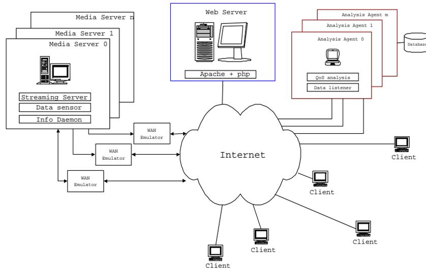
Fig. 5. Experimental system setup
