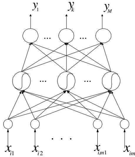
Fig. 3. A two-layer MLP neural network with one hidden layer
