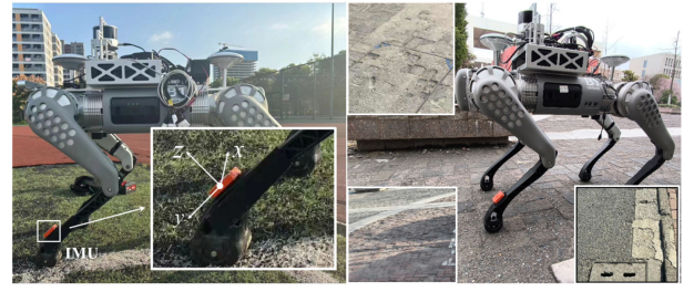
Fig. 7. Unitree B1 legged robot platform and real scenarios of Test1 and Test2.
