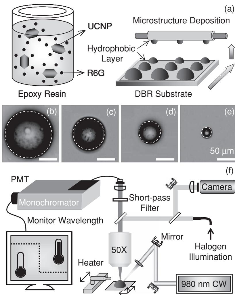
**Figure 4.** a) Schematic diagram showing the fabrication of hemispherical microstructures based on the hydrophobic effect. b–e) Top-down view optical images of microstructures with different sizes under halogen illumination; scale bars: 50  $\mu\text{m}$ . f) Schematic of experimental setup for the temperature sensing of individual microstructures. DBR=distributed Bragg reflector, PMT=photomultiplier tube.
