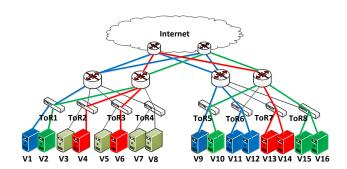
Fig. 5. Each color represent one user. Here there are totally three users. v3, v5, v7, v8 are not used by any user in this case.
