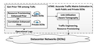
Fig. 4. The ATME architecture.
