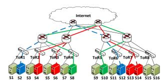
Fig. 7. Four different line styles represent four flows and three different colors represent three services.
