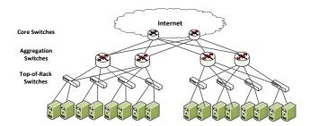
Fig. 1. An example of conventional DCN architecture, suggested by Cisco [20].
