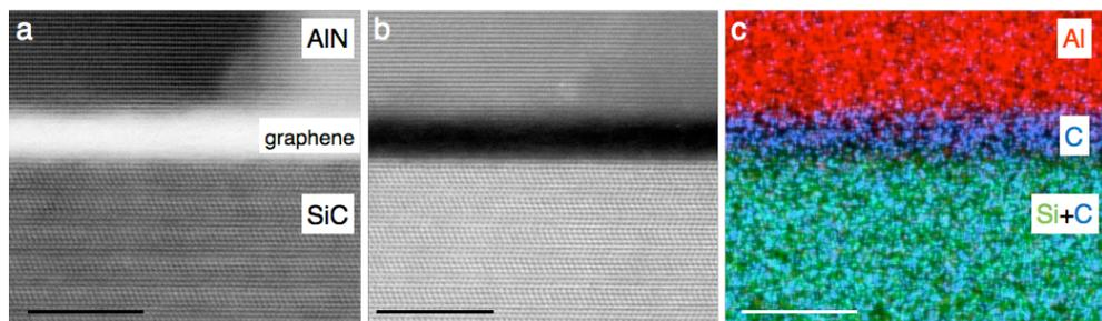
Figure 3. (a) Aberration-corrected bright-field STEM and (b) high-angle annular dark-field STEM images of the graphene layers between the SiC substrate and the AlN buffer layer. The inner ADF detector semi-angle used was 69 mrad. (c) Elemental map of Al, C and Si recorded using STEM EDXS spectrum imaging. The scale bar in each image is 5 nm.
