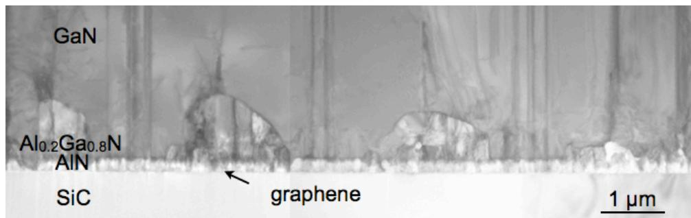
Figure 2. Low magnification bright-field TEM image of a cross-sectional specimen of the nitride heterostructure.
