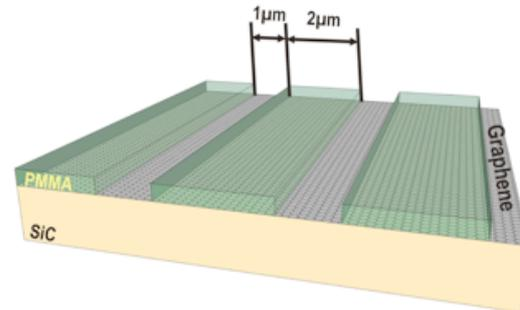
Figure 1. Schematic illustration of graphene layers patterned using PMMA.
