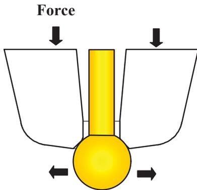
Fig. 4. A large free air ball can result in excessive gold squashed out during bonding.
