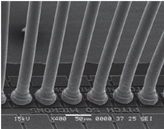
Fig. 8. An example of actual bonding responses of ultra-fine-pitch bonding on a 50- $\mu\text{m}$  bond-pad-pitch platform using  $\phi 23\text{-}\mu\text{m}$  gold wire.
