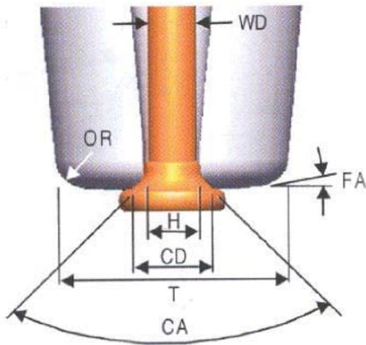
Fig. 2. Critical capillary dimensions: hole diameter (H), chamfer diameter (CD), chamfer angle (CA), face angle (FA), outside radius (OR), and tip diameter (T).<sup>18</sup>
