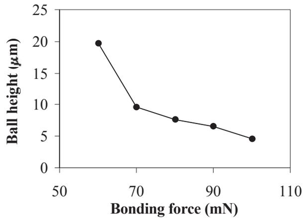
Fig. 6. The relationship between ball height and bonding force obtained by the simulation. A lower bonding force produces a thicker ball height.
