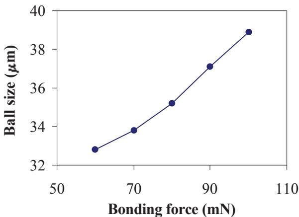
Fig. 5. The relationship between ball size and bonding force obtained by the simulation. A lower bonding force results in a smaller ball size.
