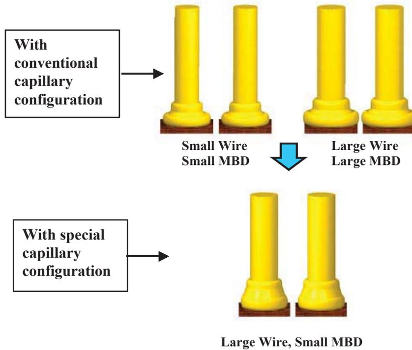
Fig. 1. A special capillary configuration produces small mashed ball diameters (MBDs) with large wires.
