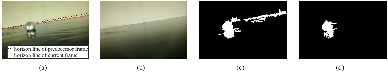
Fig. 9. Sample background subtraction outputs for the approaches with/without horizon-based image registration: (a) the original frame, (b) Gaussian component with the largest weight, (c) detection result without image registration, (d) detection result with image registration.
