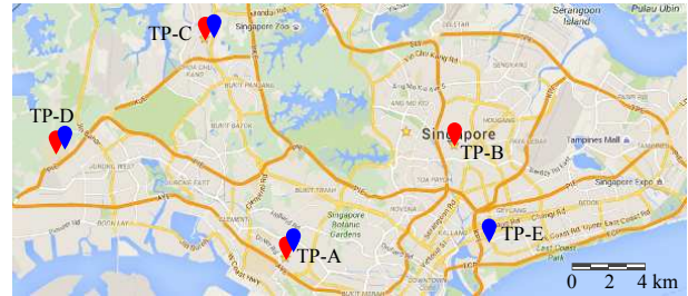
Figure 3: Sensor deployment. Red and blue markers represent voltage and EMR sensors.
