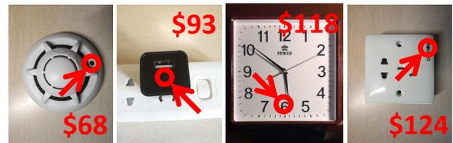
Figure 1: Examples of commodity wireless spy cameras. The arrows point to the positions of camera lens. The labeled prices are quoted from an online retailer in April, 2018 [4].
