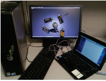
Fig. 3. Testbed for light spot detection. Four TelosB motes and a webcam detect the light spot.
