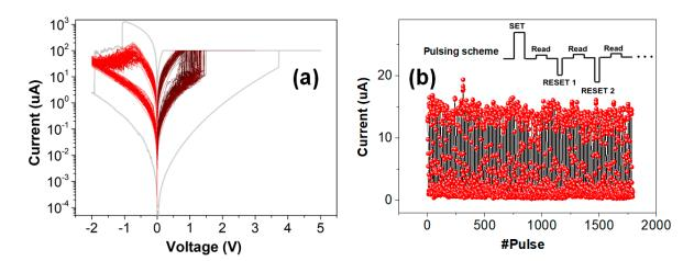
**Figure 13.** (a) DC I-V characteristics of HfO<sub>x</sub>-based RRAM device with abrupt SET and gradual RESET behavior. The grey curve indicates the forming process on the pristine device. (b) Endurance cycling performed with a single SET pulse and multiple RESET pulses (-1.2 V to -2.2 V with 0.2 V interval) for each cycle.
