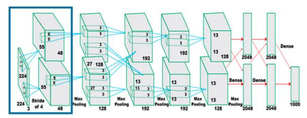
**Figure 4.** Layer 1 is a convolution layer, the input image size is  $-224 \times 224 \times 3$  (3 = RGB (8 bits each)), number of filters  $\rightarrow$  96 (Filter size  $-11 \times 11 \times 3$ ) and the layer 1 output comprises of (224/4 × 224/4 × 96 = 55 × 55 × 96) (with a stride of 4 pixels).
