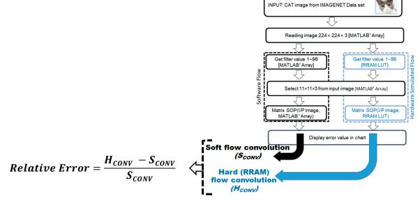
**Figure 15.** Definition of the relative error (RE) in computed matrix sum of products for the software and hardware flow convolution pipeline. The software pipeline refers to the algorithm trained weights while the hardware pipeline refers to the binary data encoded from the measured RRAM resistance distributions.
