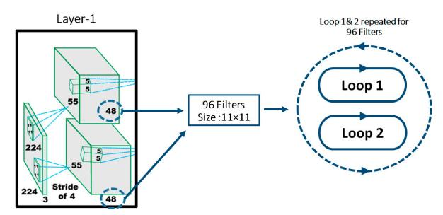
Figure 11. Total of 96 AlexNet Layer-1 filters with 48 filters each from the upper and lower pipeline.
