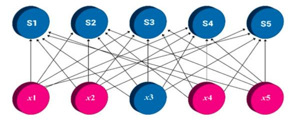
**Figure 2.** Part of the neural network architecture with a fully connected layer with input layer denoted by the nodes x1~x5 and the output layer denoted by S1~S5. Here, as an example, with matrix multiplication, all the outputs are affected by x3 (shown in blue).
