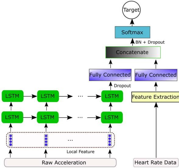
Fig. 2. Proposed framework for sleep-wake detection.
